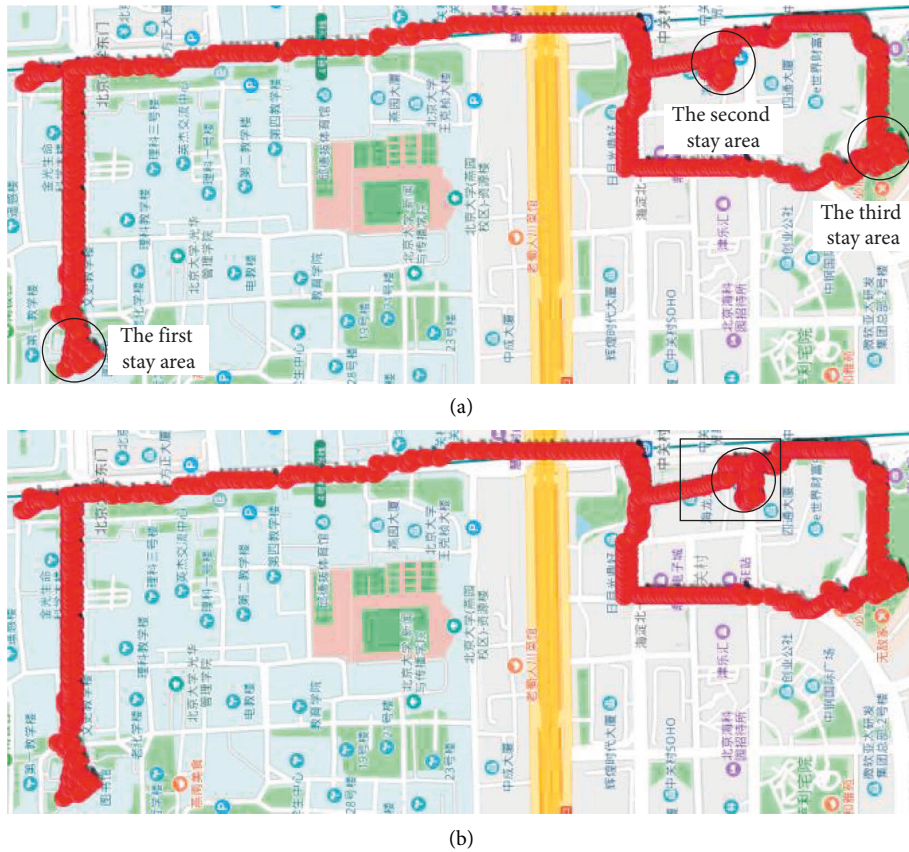
FIGURE 9: The example of practical test by SSAR. (a) The original trajectory and three stay areas(the circle). (b) The sharable trajectory, the sensitive region(the rectangular), and the replacement stay area(the circle).
