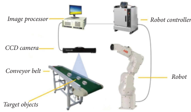
FIGURE 1: A typical conveyor belt automated production line.
