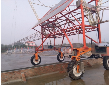
FIGURE 9: Sprinkler irrigation experiment site using the developed sprinkler irrigation machine.
