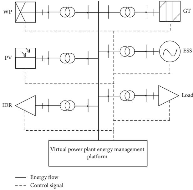
FIGURE 1: Virtual power plant structure.
