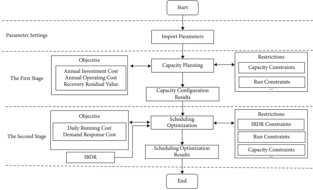
FIGURE 2: Two-stage optimization process of virtual power plant.
