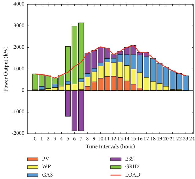
FIGURE 7: Unit output plan of typical day in transition season.
