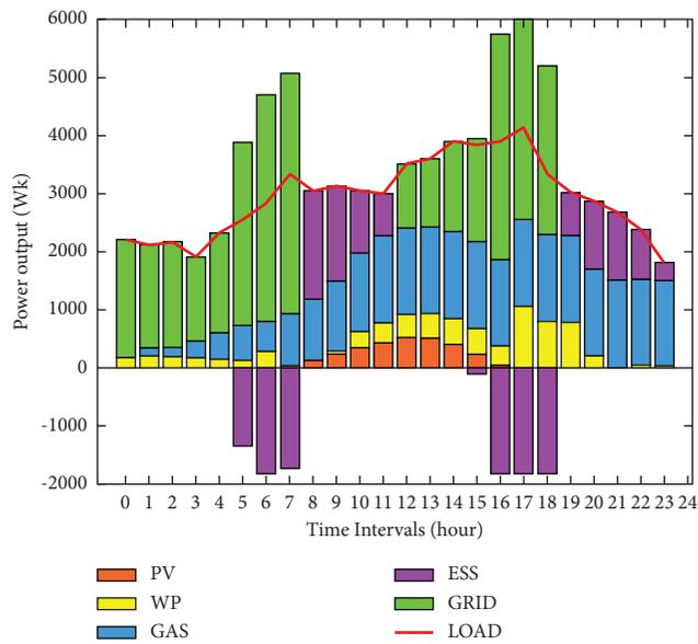
FIGURE 8: Unit output plan on typical winter days.
