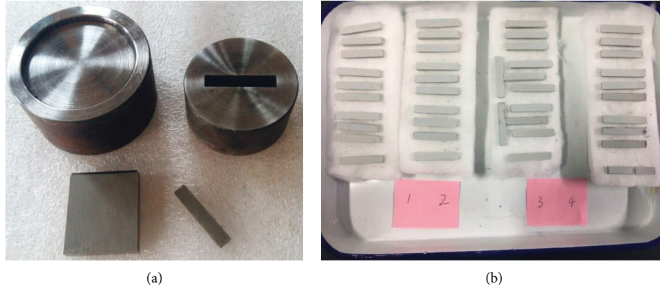
FIGURE 6: Pressing mould and green compacts of samples. (a) The special mould (b) Green compacts of SiC/Al 2 O 3 composites.
