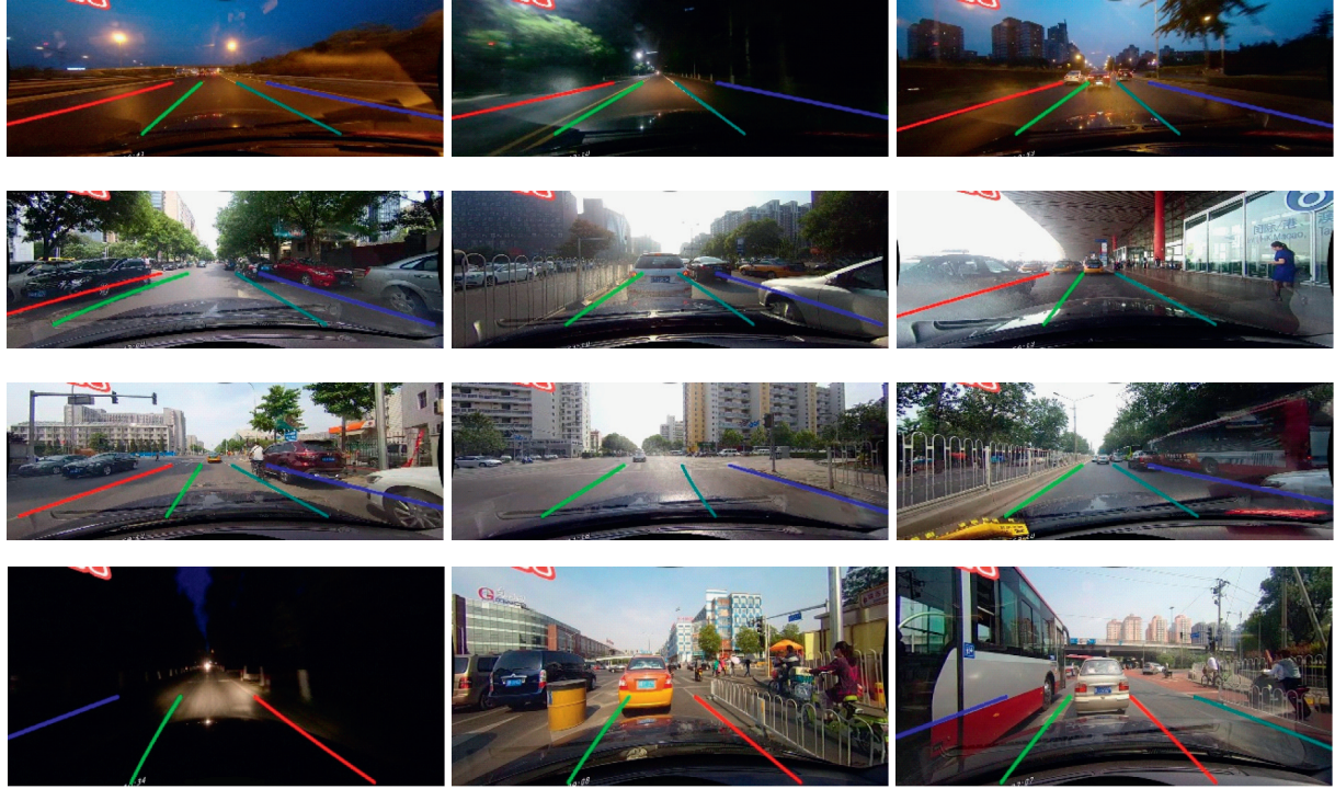
FIGURE 11: Examples of multilane line detection results.
