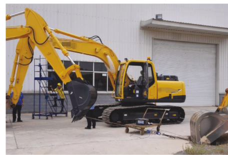
FIGURE 10: Test of maximum theoretical digging force.
