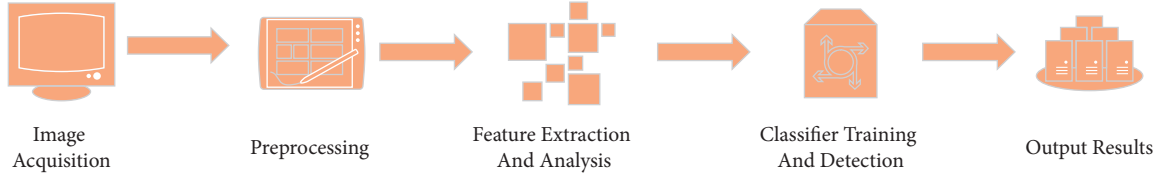
FIGURE 4: Main flow of the system.
