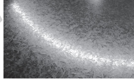
FIGURE 1: Machining workpiece surface (200x). \nu = 280 m/min, f = 0.08 mm/r, and a_p = 0.2 mm.
