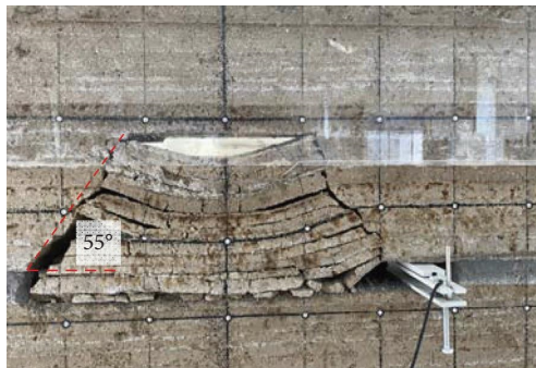
FIGURE 3: The first caving of main roof.
