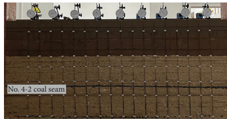
FIGURE 7: Physical simulation experiment model of Hongliulin Coal Mine.
