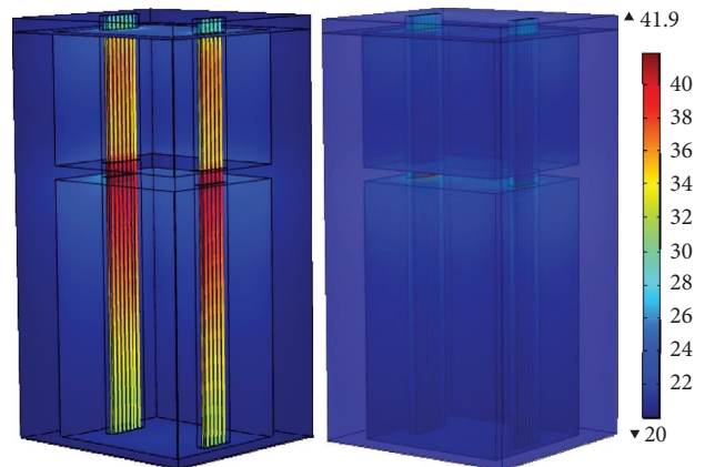
FIGURE 10: Thermal distribution inside the cable shaft (with firestop material).
