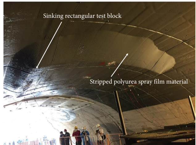
FIGURE 24: The condition of the cuboid test block after sinking.
