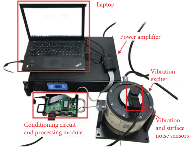
FIGURE 8: Setup of the test bench for standard vibration signal measurement.
