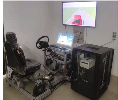
FIGURE 6: Hardware-in-the-loop test platform.
