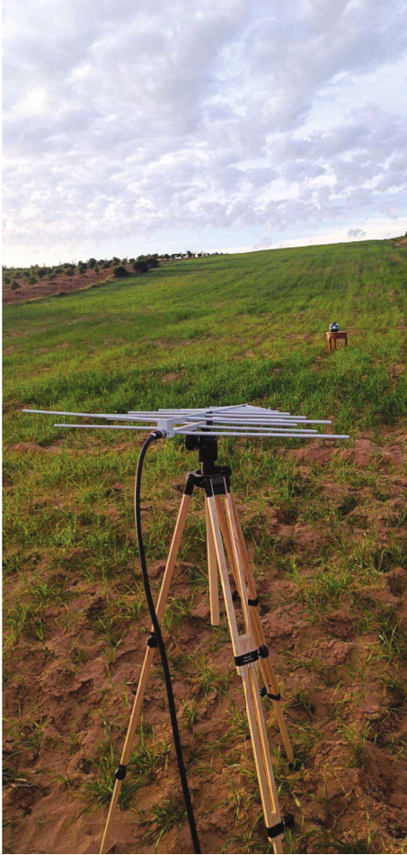
FIGURE 4: Radiated emission in open test area (10 m between the transmitter TX and the receiver RX).
