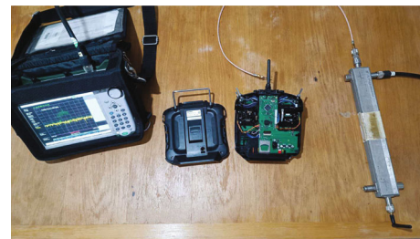
FIGURE 2: Conducted emission measurement of the transmitter T14SG.
