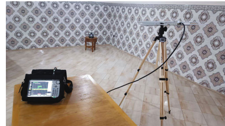
FIGURE 3: Radiated emission measurement in the laboratory basement (4 m between the transmitter TX and the receiver RX).
