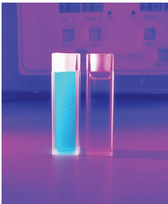
FIGURE 10: The recorded fluorescence images of a CQD solution before (left) and after (right)  $\text{Cu}^{2+}$  ion addition at room temperature.
