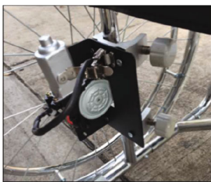
FIGURE 3: The electric motor of the prototype for the simplified power wheelchair.
