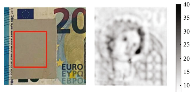
FIGURE 8: Images of the watermark included in a 20 EUR banknote obscured by a metallic mask [42].
