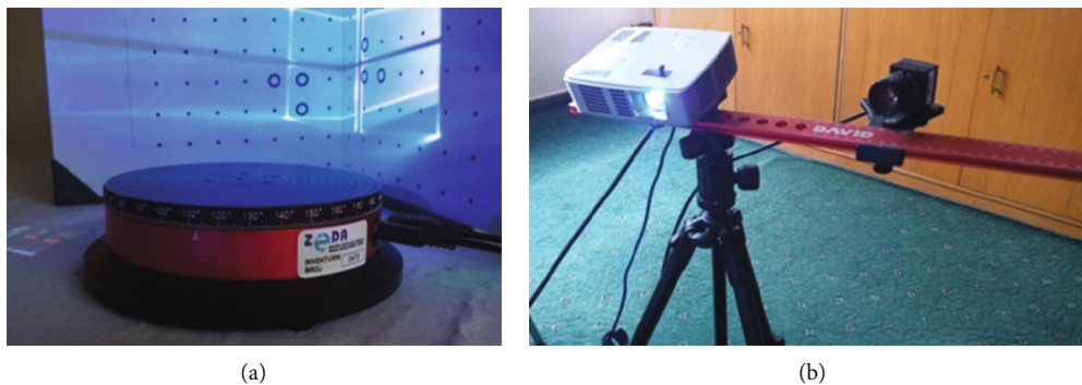
FIGURE 1: HP 3D Structured Light Scanner Pro S2 Laser Scanner (DAVID SLS-2); camera, projector, and stand (b); calibration plate and rotating stand (a).
