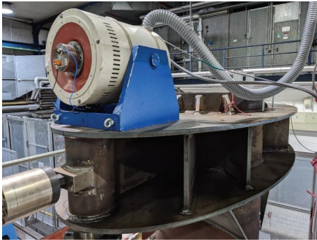
FIGURE 4: Electrodynamic shaker used for dynamic testing during the fatigue test.
