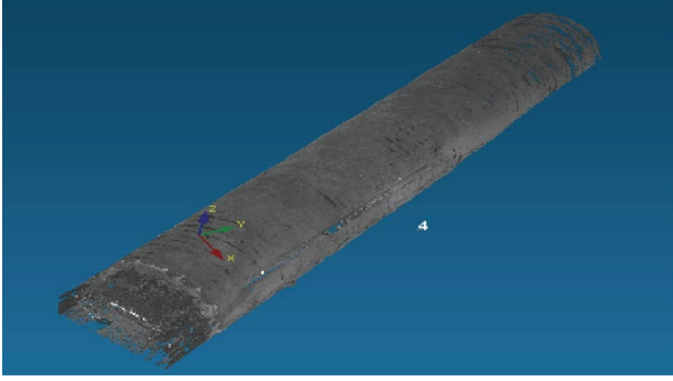
FIGURE 7: Overall drawing of the tunnel point cloud.
