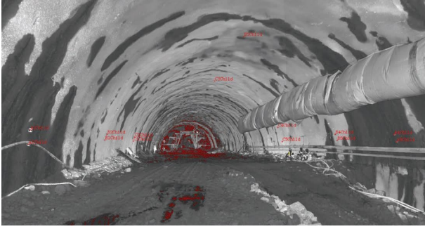
FIGURE 6: Monitoring measurement point cloud measured grayscale image.
