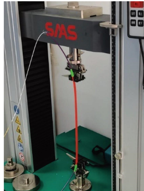
FIGURE 3: Tensile calibration test of DFOS.
