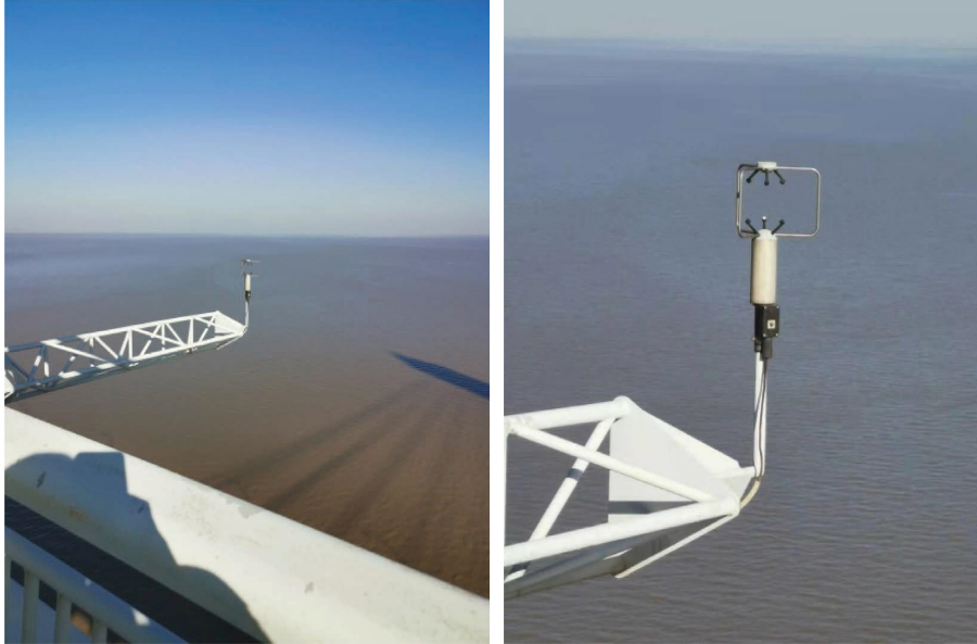
FIGURE 2: Deployment of wind anemometers on the investigated bridge.
