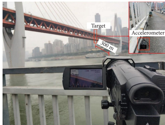
FIGURE 42: Overview of the cable-stayed bridge test.
