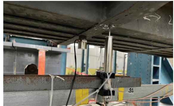
FIGURE 18: Accelerometer and LVDT.
