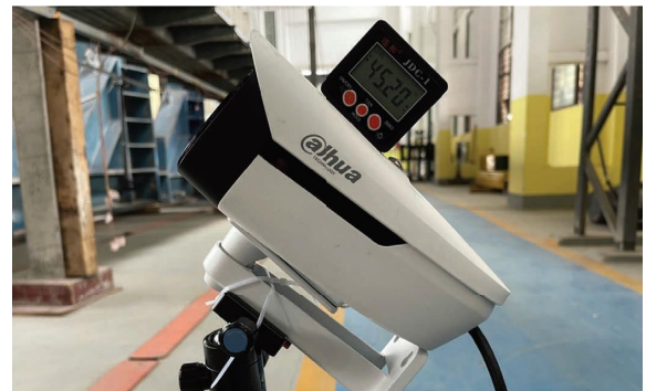
FIGURE 19: Tilted camera and angle measurement.
