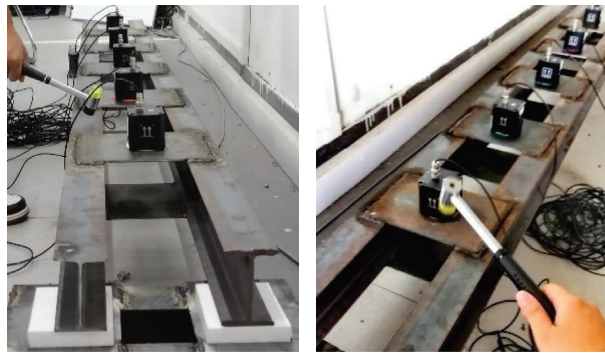
FIGURE 10: Test structure subjected to pulse excitation.
