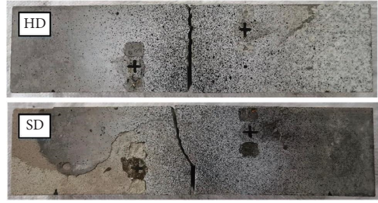
FIGURE 12: Fracture morphology of HD and SD specimens.
