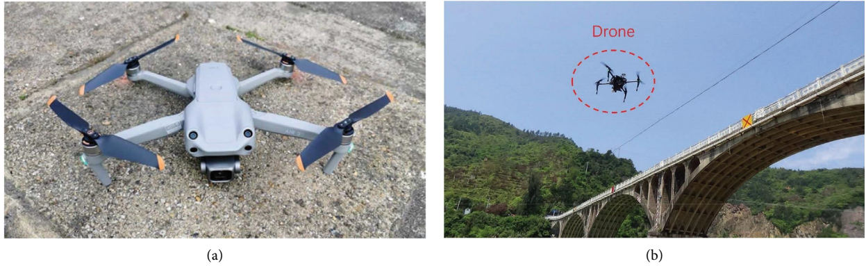
FIGURE 6: Carrying out bridge inspection based on UAV detection technology. (a) UAV-based inspection equipment equipped with cameras. (b) UAV-based bridge damage detection.
