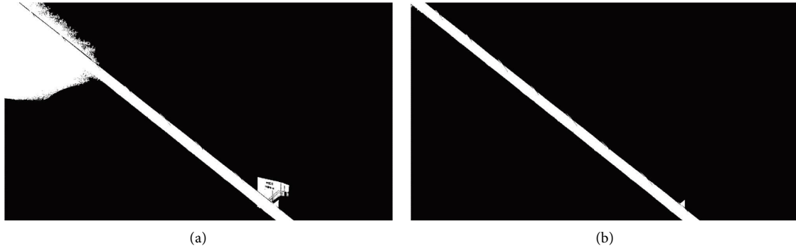
FIGURE 7: The effect of tuning parameters in the Region Growing algorithm. (a) The gray threshold is set to 0.25; (b) the gray threshold is set to 0.20.
