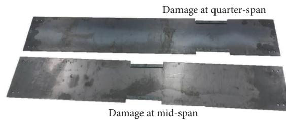
FIGURE 13: Created artificial damage in the bridge.
