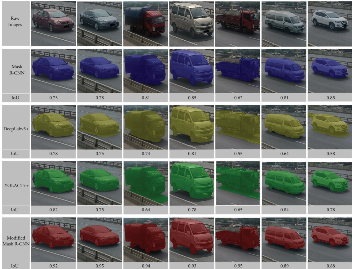
FIGURE 14: Comparisons of the original Mask R-CNN, YOLOACT++, DeepLabv3+, and modified Mask R-CNN for segmenting vehicles from images with complex traffic backgrounds.
