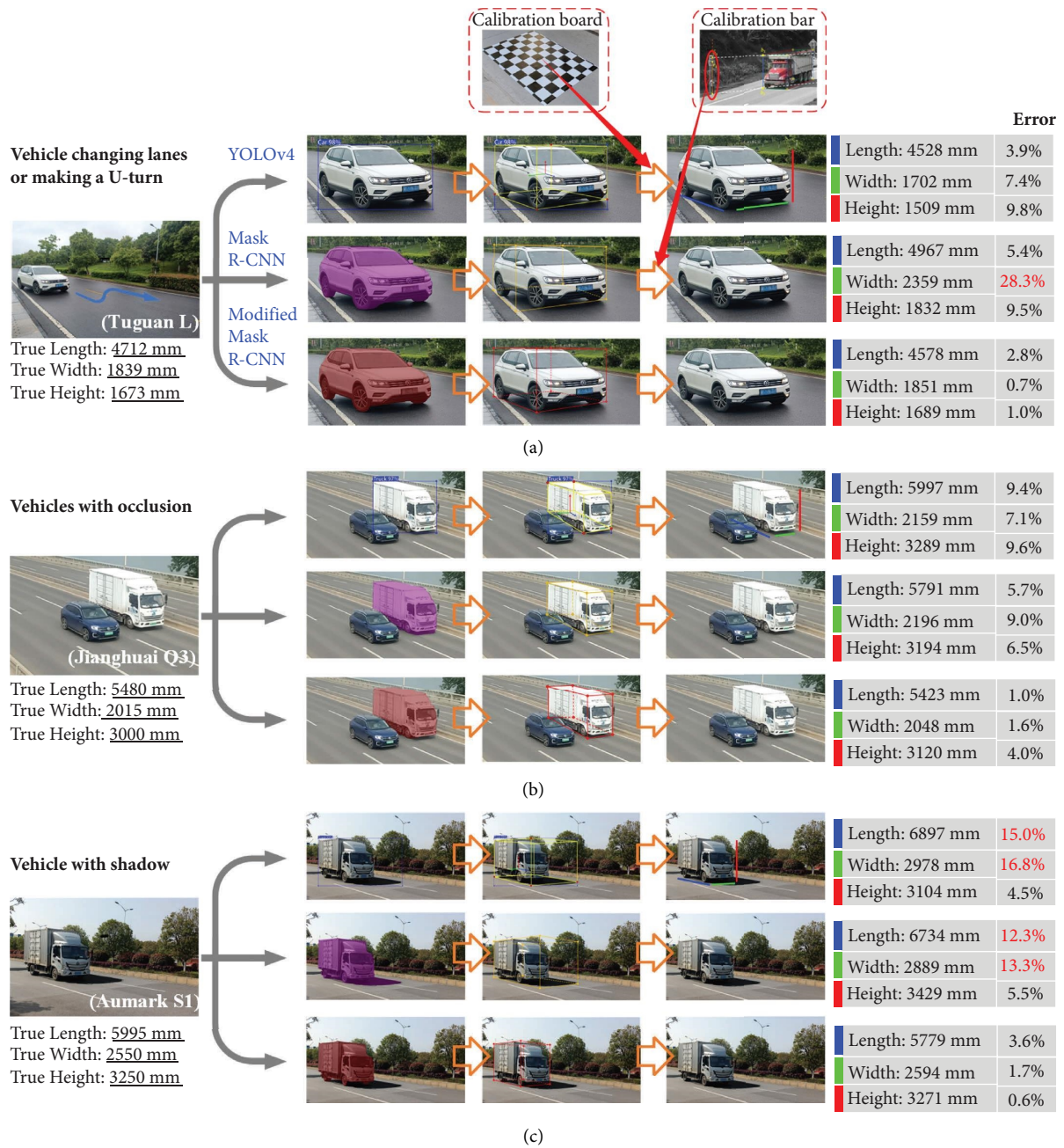
FIGURE 17: The results of identifying vehicles' dimensions in special traffic situations using three methods: (a) vehicles are changing lanes or making a U-turn; (b) there is occlusion between vehicles; (c) there is shadow interference around vehicles.
