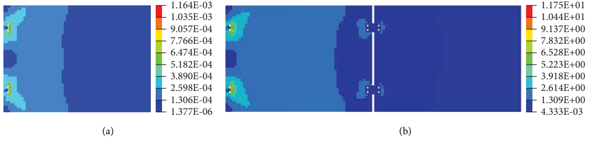
FIGURE 3: The strain energy distribution of the first-order vibration mode of the solar array. (a) The strain energy distribution of the first-order vibration mode of the single-board solar array. (b) The strain energy distribution of the first-order vibration mode of the double-board solar array.
