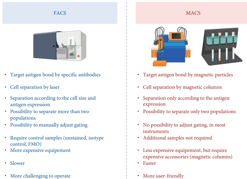
FIGURE 2: Fluorescence-activated cell sorting (FACS) and magnetic activated cell sorting (MACS)—properties comparison. Abbreviation: FMO: fluorescence minus one.
