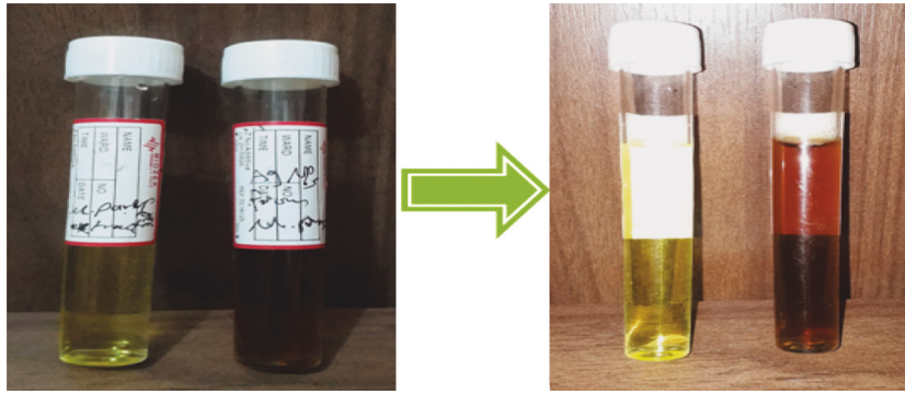
FIGURE 4: Color change during the reduction process for biosynthesis of AgNPs.
