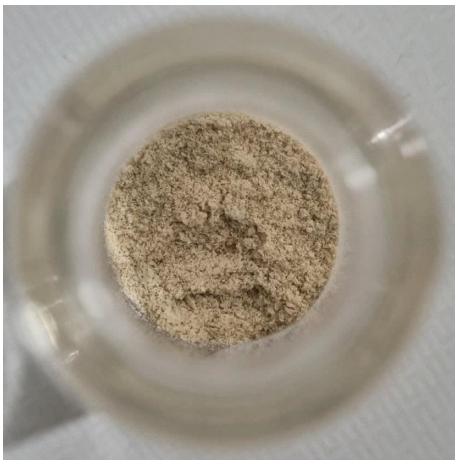
FIGURE 4: Microcapsules powder from the combination of R. tuberosa L. and T. diversifolia extract prepared in pH 5, 4% (w/v) gum Arabic, and 60 min stirring time.
