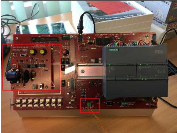
(a) The Siemens S7-1200 PLC with the motor and HMI connection outlined
