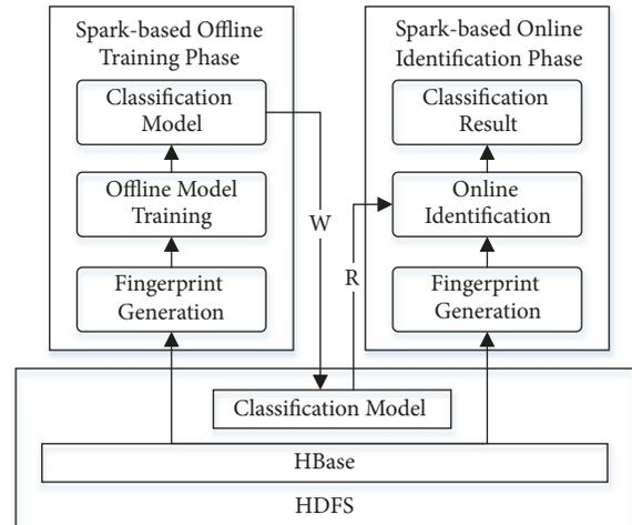
FIGURE 3: Two-stage fingerprint recognition.
