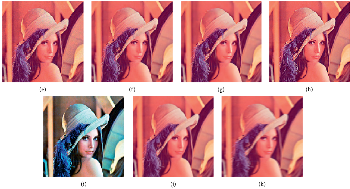
FIGURE 8: Various attacks on watermarked images. (a) Gaussian low-pass filter, (b) median, (c) Gaussian noise, (d) salt and pepper noise, (e) speckle noise, (f) JPEG compression, (g) JPEG2000 compression, (h) sharpening attack, (i) histogram equalization, (j) average filter, (k) motion blur.
