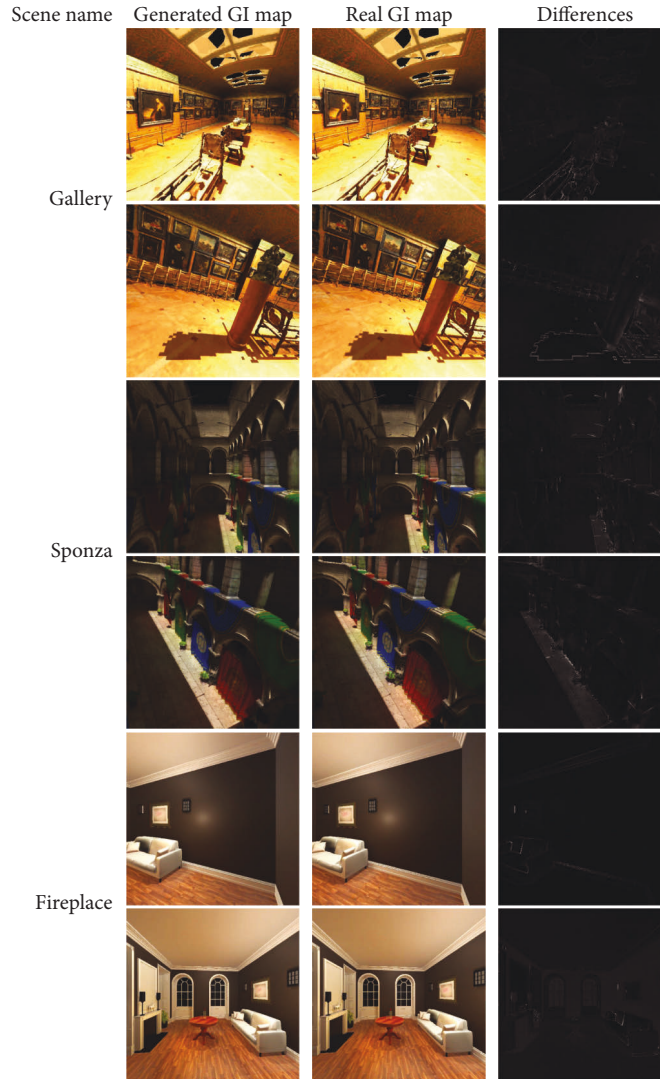
FIGURE 8: Generated GI map VS. Real GI map. The difference between the differential GI map and the Real GI map pixel-by-pixel difference operation can be more intuitively recognized. The darker the color, the smaller the difference between the corresponding pixels. These results show that the generated GI maps are very close to the real GI maps.
