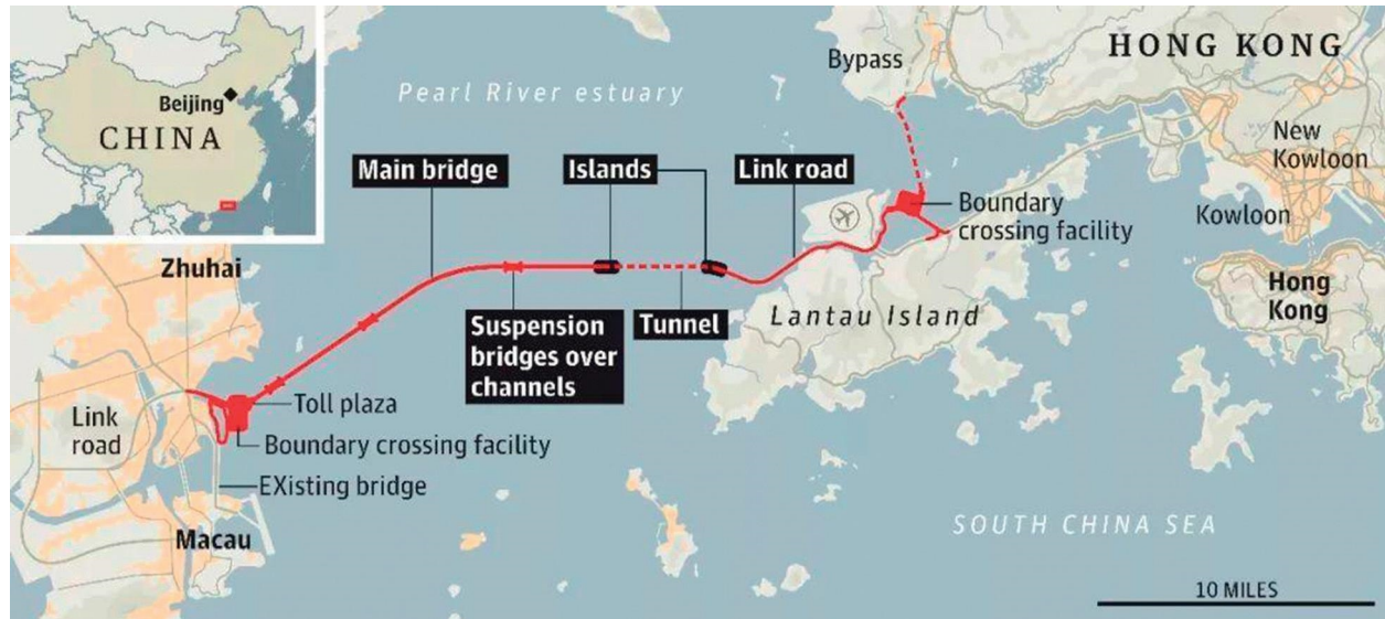
FIGURE 1: The spatial structure of the Hong Kong-Zhuhai-Macao Bridge.
