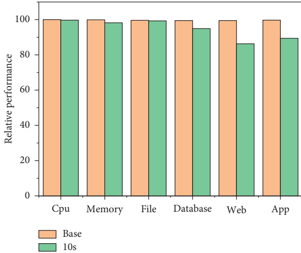
FIGURE 2: Impact of DIMA runtime reliability on the performance of benchmark test set.
