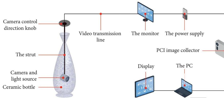
FIGURE 1: Structural diagram of ceramic bottle crack detection system.
