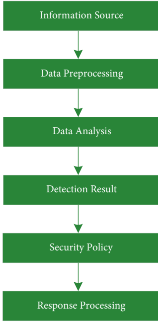
FIGURE 2: Process of intrusion detection.
