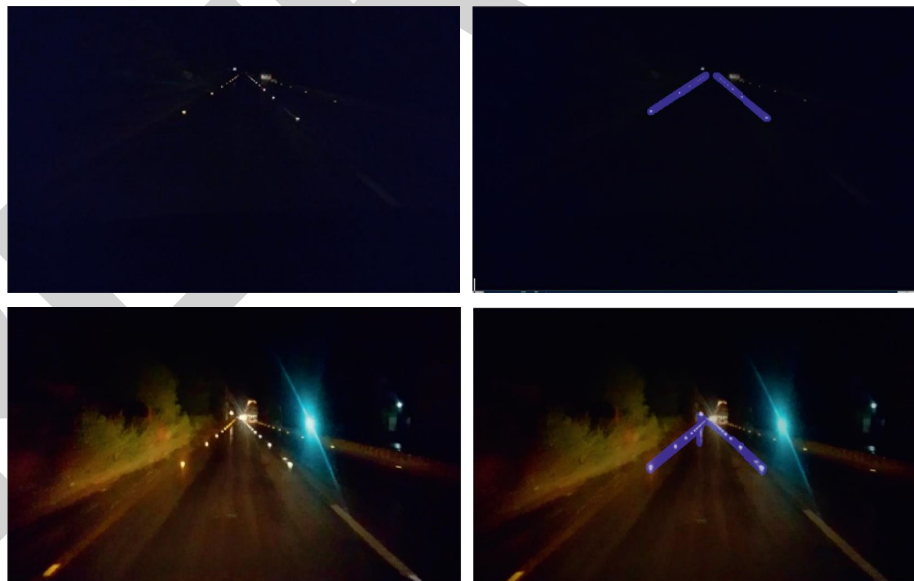
FIGURE 15: Sample results of the proposed stud detection algorithm before and after preprocessing.
