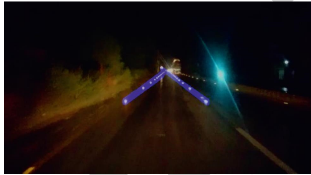
FIGURE 14: The stud detection result of the proposed approach after employing the Hough transform.
