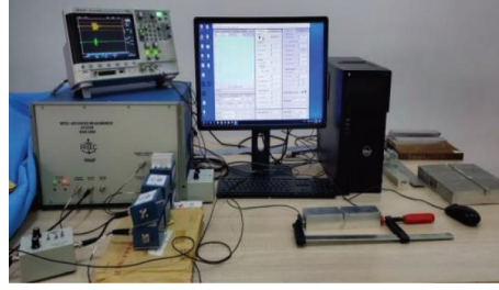
FIGURE 7: Experimental platform setup of nonlinear Lamb detection.
