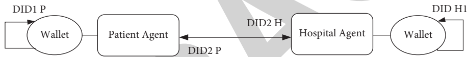
FIGURE 6: Establishing a mutually authenticated channel between the patient and the hospital by creating pairwise DIDs for this specific relationship.
