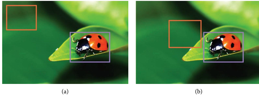
FIGURE 7: Different scenarios when IoU is 0. (a) The prediction frame is far away from the real frame. (b) The prediction frame is closer to the real frame.
