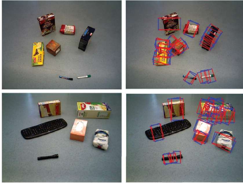
FIGURE 7: Performance of our model on the OCID dataset. In the output bounding box, the red line represents the open length of a two-fingered gripper, while the blue line represents the parallel plates of the gripper.
