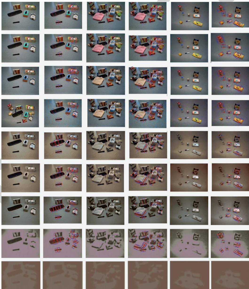
FIGURE 17: The first line is the result of the grasp detection of the original image, and the lines below are the results under the compression ratio of 16.29%, 4.07%, 0.99%, 0.5%, 0.13%, 0.05%, 0.04%, and 0.03%. From top to bottom, the loss of pictures due to compression gradually increases, which slowly affects the bounding box results of grasp detection.
