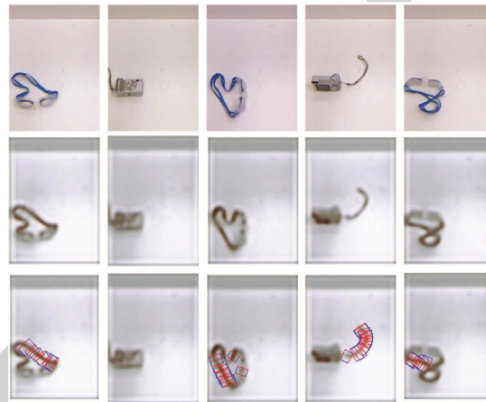
FIGURE 14: Grasp detection result under 0.06% compression ratio. The loss of image reconstruction becomes large, and some objects cannot be correctly recognized.
