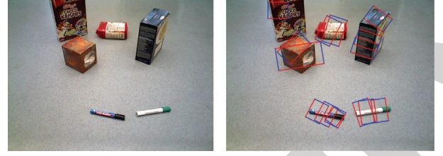
FIGURE 4: Results of grasp detection output. The red line represents the open length of a two-fingered gripper, while the blue line represents the parallel plates of the gripper.
