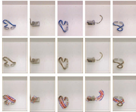
FIGURE 13: Grasp detection result under 0.13% compression ratio. The image is blurred, but it can still be used for grasp detection.
