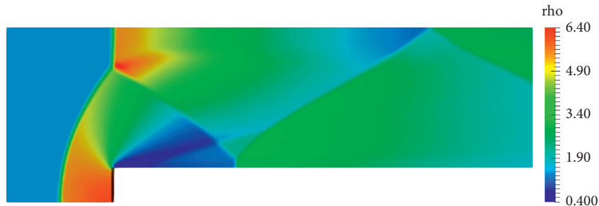
FIGURE 2: Density distribution in supersonic forward facing step simulations obtained using rhoCentralRK4Foam.
