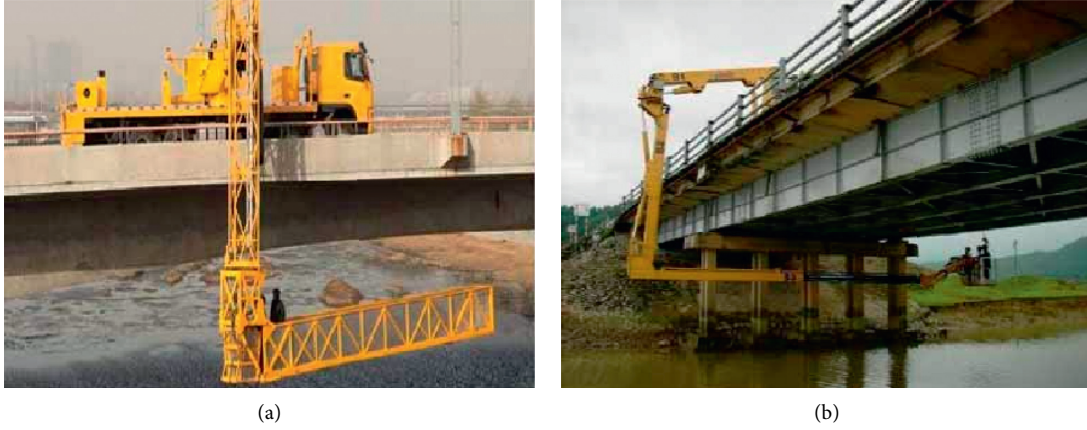
FIGURE 3: Example of a bridge inspection vehicle. (a) Truss-type bridge inspection vehicle. (b) Basket type bridge inspection vehicle.
