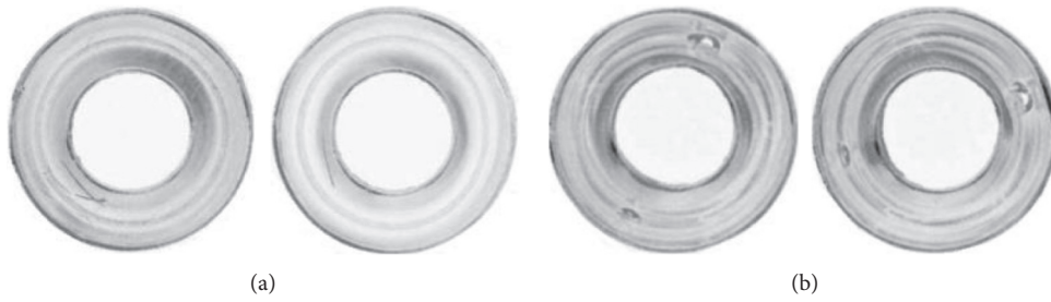
FIGURE 4: B component image of the RGB image. (a) Scratches. (b) Melting point.
