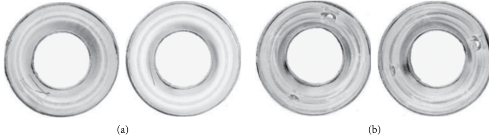
FIGURE 5: The filtered image. (a) Scratches. (b) Melting point.
